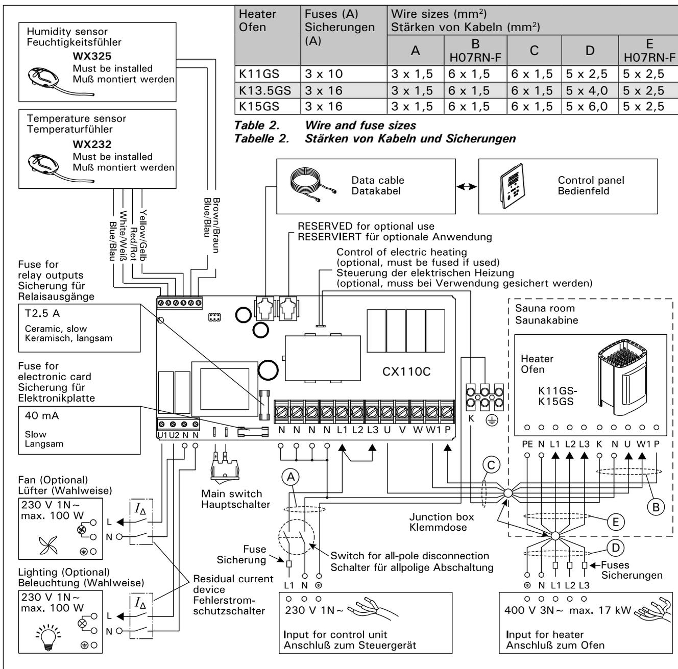
**Figure 6. Electrical connections (K11GS–K15GS)**
