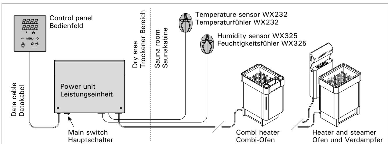
Figure 1. System components
